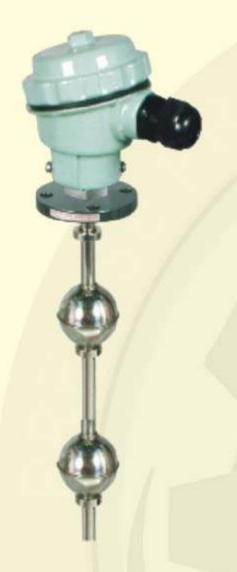
A Top Mounted Magnetic Level switch is normally a simple device that monitors the liquid level in a tank and sends a trip signal to another device such as a Pump to protect it. These Level switches are used for Pump protection, Cooling Circuit protection, high & low level alarm and general level monitoring.
